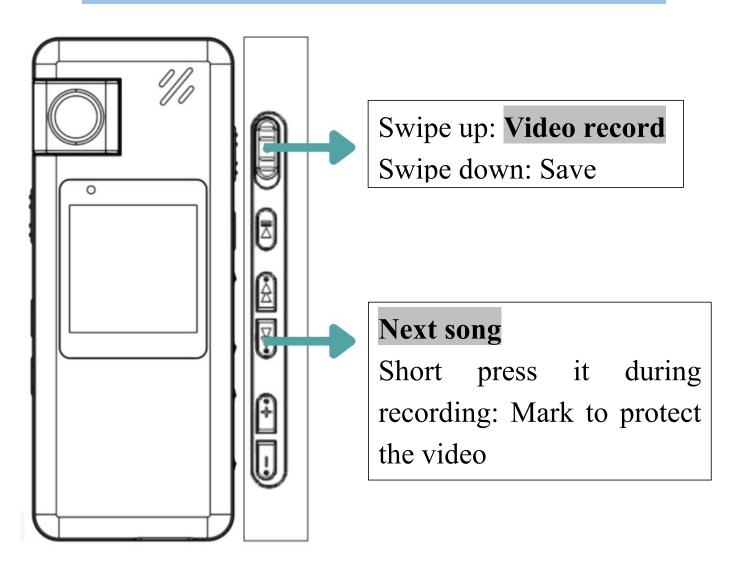
**Note:** To avoid losing files for too large, video files are automatically saved as one file for 10 minutes. Short press "Back" button to turn off the screen when recording
